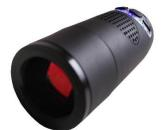
MICFIEYE is a USB & Wi-Fi camera with C-mount and allows to digitalize the image on tablets, smartphones and Pc using dedicaded Apps and Softwares that allow to capture photo, video and measurement (only when the camera is connected with a optical microscope). MICFIEYE is compatible with all optical devices such as microscopes, endoscopes, boroscopes, fiberscopes, c-mount lenses etc.
